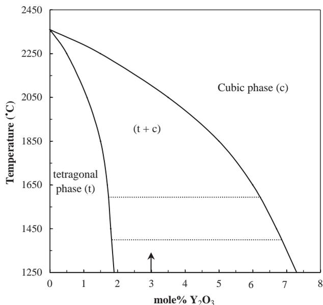
Fig. 1. Selected region of the  $ZrO_2$ - $Y_2O_3$  equilibrium phase diagram (after Scott [15]). The dashed lines show the typical range of sintering temperatures of 3 mol % yttria-stabilized zirconia.
