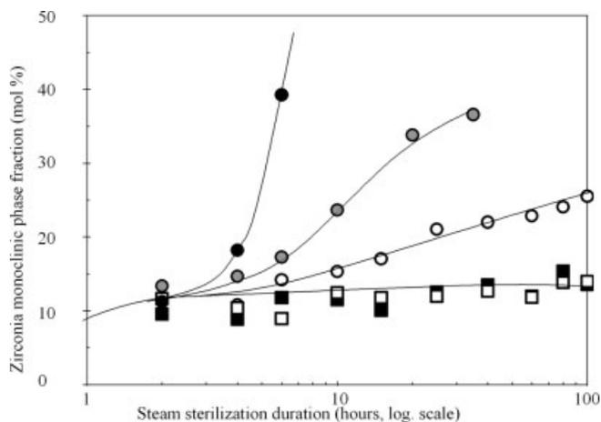
Fig. 3. Fraction of monoclinic phase vs time of steam sterilization for alumina/3Y-TZP composites with different zirconia content. □: 7 vol.-% zirconia, ■: 14 vol.-%, ○: 22 vol.-%, ●: 40 vol.-%.
