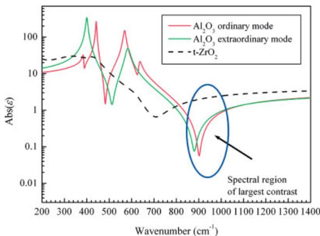
Fig. 1. Absolute value of the dielectric constant for the ordinary ( $E_u$ ) and extraordinary ( $A_{2u}$ ) modes of alumina and tetragonal zirconia.
