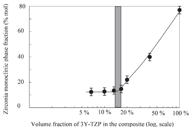
Fig. 5. Fraction of monoclinic phase measured after 40 h steam sterilization as a function of the zirconia volume content in the composite. The dashed area represents the percolation threshold measured by IR study.
