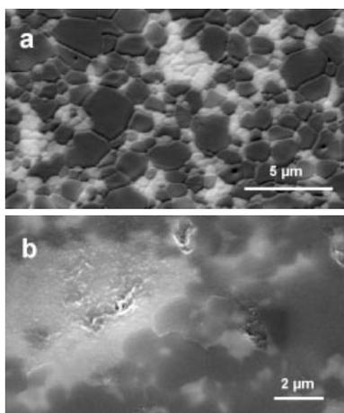
Fig. 4. SEM micrographs of polished surface of alumina/22 vol.-% 3Y-TZP a) before and b) after 115 h steam sterilization.
