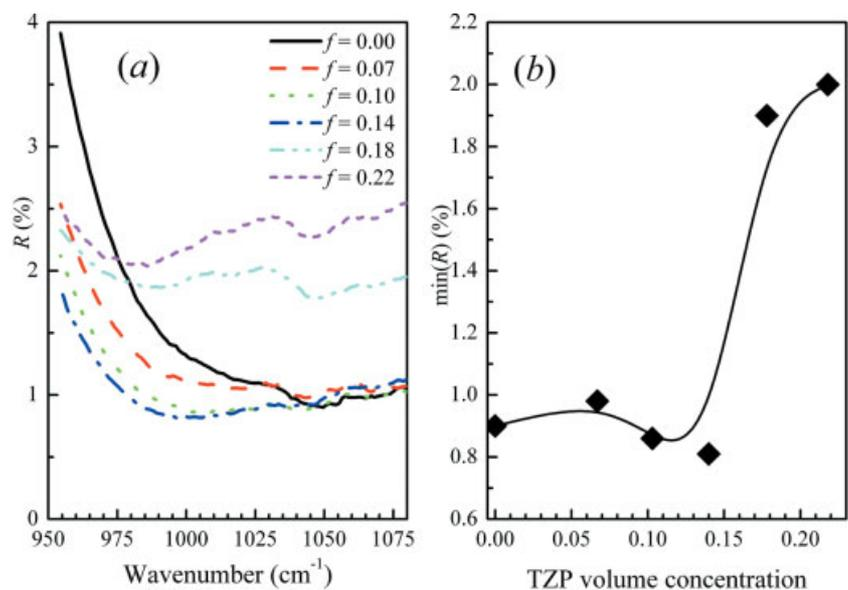
Fig. 2. a) Near-normal reflectance spectra of alumina/3Y-TZP composites in the region of the minimum of reflectance. b) Minimum of reflectance vs 3Y-TZP volume fraction ( $f$ ). The solid lines are guides to the eyes.
