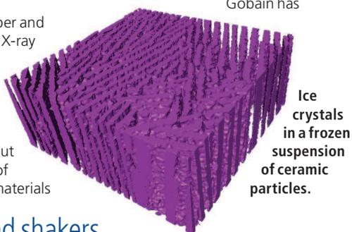
Ice crystals in a frozen suspension of ceramic particles.
