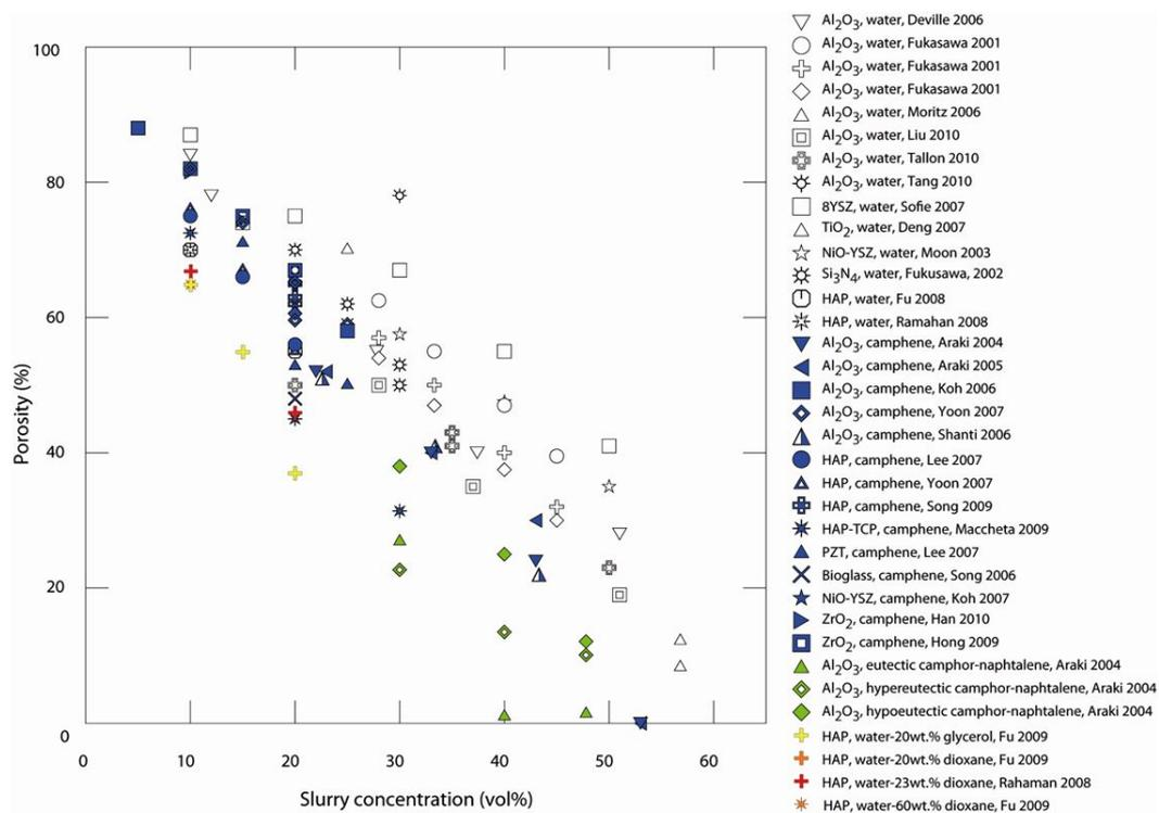
Figure 1: Total porosity vs. slurry concentration, literature data<sup>2,8-31</sup>. The samples made with water, and camphene are respectively in white and dark. Other solvent are also represented, although fewer results can be found. The porosity of samples made with camphene is almost systematically lower than when made with water.
