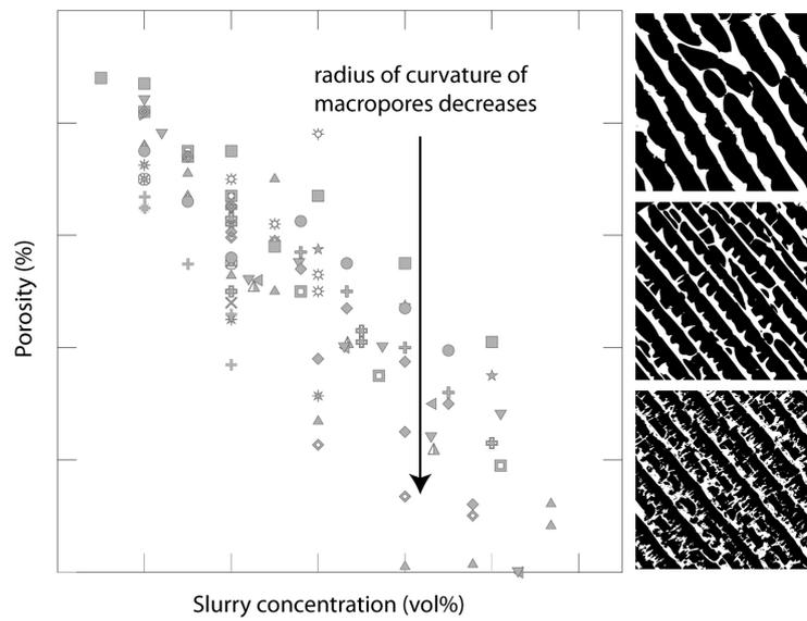
Figure 4: Total porosity vs. slurry concentration. The decrease of porosity, for a given slurry concentration, corresponds to a decrease of the radius of curvatures of the macropores, with typical structures schematically shown on the right.
