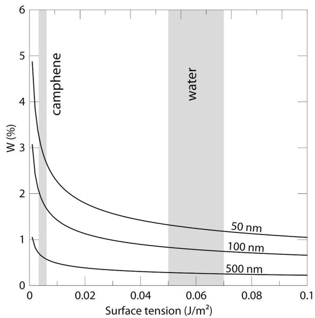
Figure 2: W vs. surface tension, for various particle sizes, and for a fixed temperature of 273K. The surface tension of water is very sensitive to the presence of impurities and usually lower than the value for pure water.
